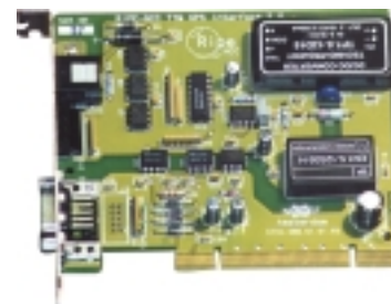
Interface board for the Trimble GPS receivers, developed in collaboration with NIKHEF
