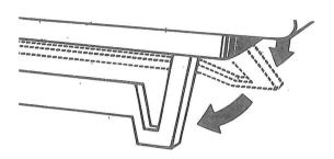
You can tilt the monitor into a convenient position with regard to the computer by using the movable support.
