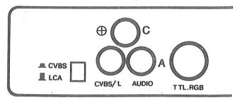
CVBS/L (Luminance) IN (Phono type) CVBS (composite signal) or Luminance input Phono plug type. For connection of a computer or other CVBS sources.
