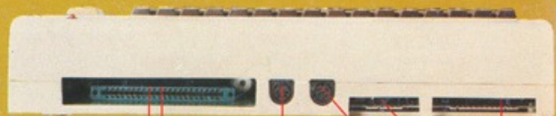
PLUG-IN PROGRAMS 32K/16K MEMORY EXPANSION EXPANSION MODULE RF MODULATOR TELEVISION OR MONITOR VIDEO CABLE SINGLE DISK DRIVE PRINTER COMMODORE DATACASSETTE MODEM FOR TELEPHONE AND TELECOMPUTING
