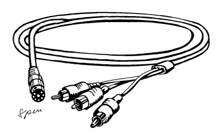
If you intend to connect either composite or monochrome, you will need a different cable. Composite mode, which can be used to display the picture from a television tuner or VCR, needs a cable with only two phono plugs to connect, or you can use multi-purpose male phono patch cables. To connect monochrome properly, you may
