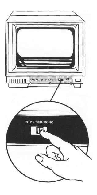
**To connect the monitor for COMPOSITE display**, you'll need either a five-pin cable with two plug ends (instead of three) or RF cables to hook up composite from a computer, VCR or TV tuner.
