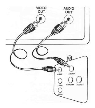
3. Set the VIDEO MODE SWITCH to COMP (for composite) to view computer or video output in a 40-column color picture display.
