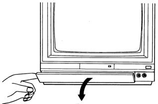
This panel is flipped down by pulling it towards you as shown in the diagram.
