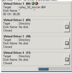
notice the virtual driver has changed and shows a green on and a red loading light, the c64 hardware shows 1 amber light and this denotes the c64 is loading from disk this took around 2 mins to load notice on the pc you see a real-time progress bar
