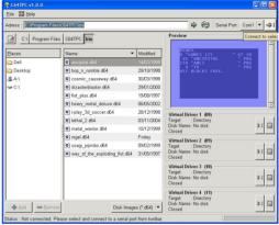
click on the serial icon it should read connect to selected device ensure your coms port is selected default is com 1 on the pc this should be labelled up com1 or com2 most modern pcs will just have a com1 or only usb so you need a usb to seral port adaptor although I don't think this has been tested!
