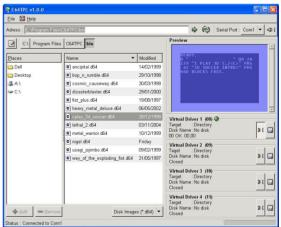
you notice the green light goes on and the device plugged into the c64 changes the amber lights go out and the green light comes on the device is ready and connected. you also see that the preview displays what is in the d64 file on the pc preview window now mount the disk by clicking on the disk button
