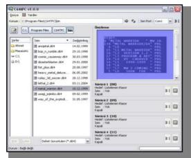
course consists of the two components: an electonic device and a PC software. The electronic device solves low level process for communication between C64 and PC. Thus, user does not need to struggle with complex settings or processes. C64TPC's software is a program with graphical user interface for simply usage. I will be able to release the binary for GNU/Linux and MacOS X because its source codes is platform independent.
