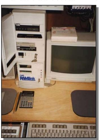
Installed in the tower are a Ramlink; a CMD FD 4000; a CMD Hard Drive; and a 14.4 modem attached to a SwiftLink.
