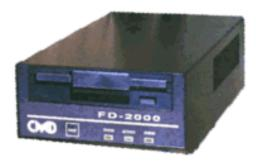
The device is a 3.5 1581 clone however it adds the bonus of being able to use high density disks, making this device very useful for the casual Commodore user. Has jiffy dos on the device. Also can Swap device numbers with attached disk drives
