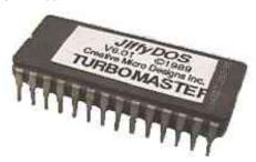
Jiffy dos is a floppy drive speed up system the chip needs fitting in the Commodore machine and also in your drives for the device to function to its potential, but as the ram link SCPU and FD drive have jiffy dos already installed, you could add a SCPU and a FD200 disk and be jiffy dos enabled, although other disk drives will need the chip fitted to take advantage
