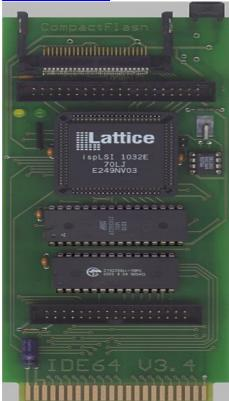
The ide 64 is a cartridge that allows standard pc IDE disk and cd rom drives to be connected to your Commodore, although it seems everyone is sold out there is a new version in the making see this link for more details <a href="http://www.ide64.org/ide64v4.html">http://www.ide64.org/ide64v4.html</a>
