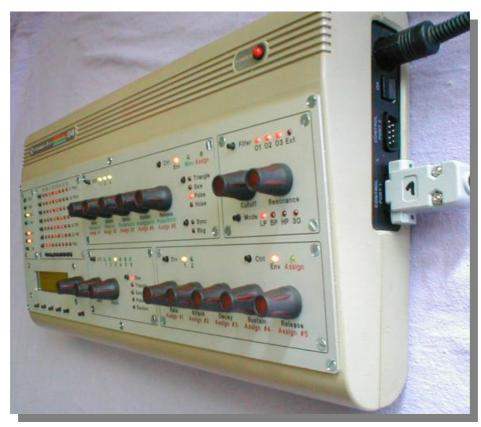
Both of these projects are based on the classic **MIDIbox** SID, which converts the C64's beloved SID synth chip into a usable MIDI interface. complete with interface, friendly knobs, and lots of flashing lights. (Thanks to Wisefire for pointing this
